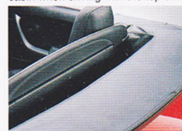
A new design was developed for the Windblocker™ to keep wind out the cabin when driving with the top down.
