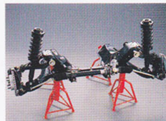
The tuned, 4-wheel double wishbone suspension resulted from testing many different combinations of handmade parts.
